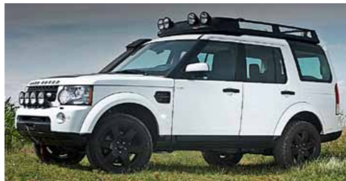
3 Matzker switch Position 2: Standard on-road ride height +30mm for on-road speeds on rough desert tracks or wide open terrain – perfect for touring North Africa or Mongolia.
