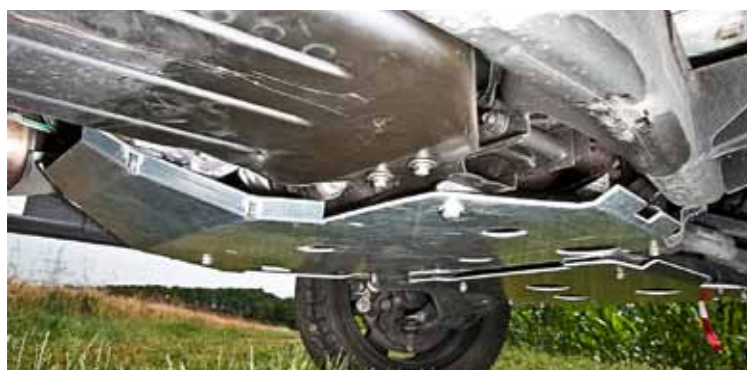
Robust 6mm steel belly plate incorporates strategically placed servicing 'holes'
