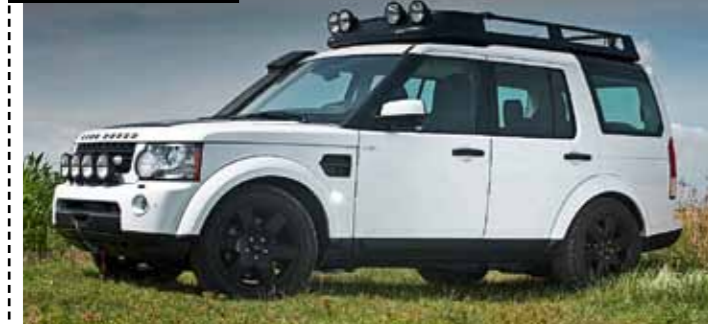
1 Matzker switch Position 1: 25mm lower than standard on-road height. Not as low as access height. Perfectly designed for high-speed autobahn cruising, reducing effects of side winds.
