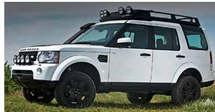
4 Matzker switch Position 2: Standard off-road height +30mm for maximum off-road clearance up to 45kph, at which point it will drop by 55mm but will still be 30mm higher than standard.
